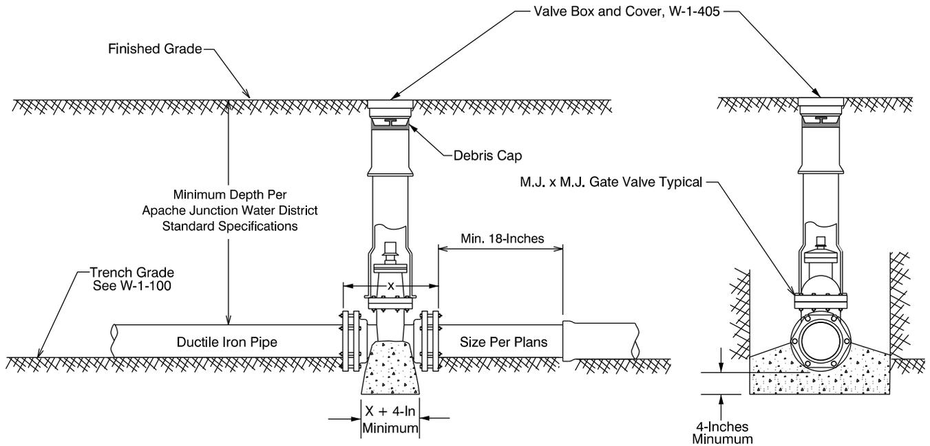
Form as Required to Keep Clear of Joints and Bolts
