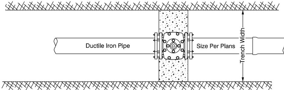
Valve operator extensions are required on all valves when the operating nut is over 5-feet below finished grade. Extensions will bring the operating nut within 24 to 36-inches of the top of the valve box. Extensions will be steel with a centering collar and 2-inch operating nut as manufactured by Pipeline Products, Part No. SX-906. Length as required.
