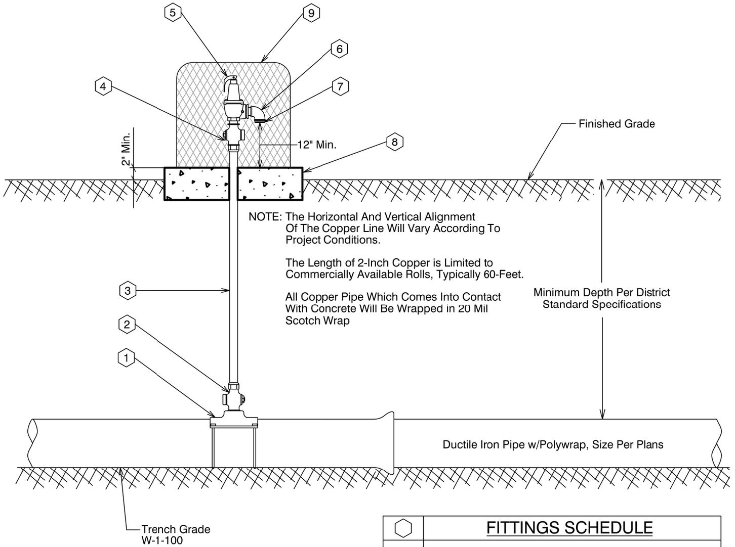
NOTE: The Horizontal And Vertical Alignment Of The Copper Line Will Vary According To Project Conditions.
