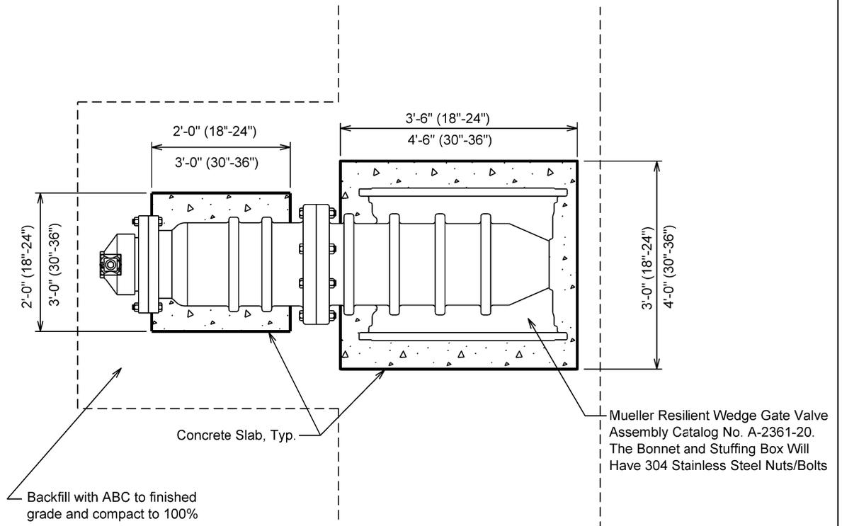
All concrete slabs to be class "C", which is defined as concrete whose minimum compressive strength at 14 days reaches 1600psi and at 28 days reaches 2000psi, per MAG Section 725, Table 725-1. Slabs to be formed and poured prior to valve installation.
