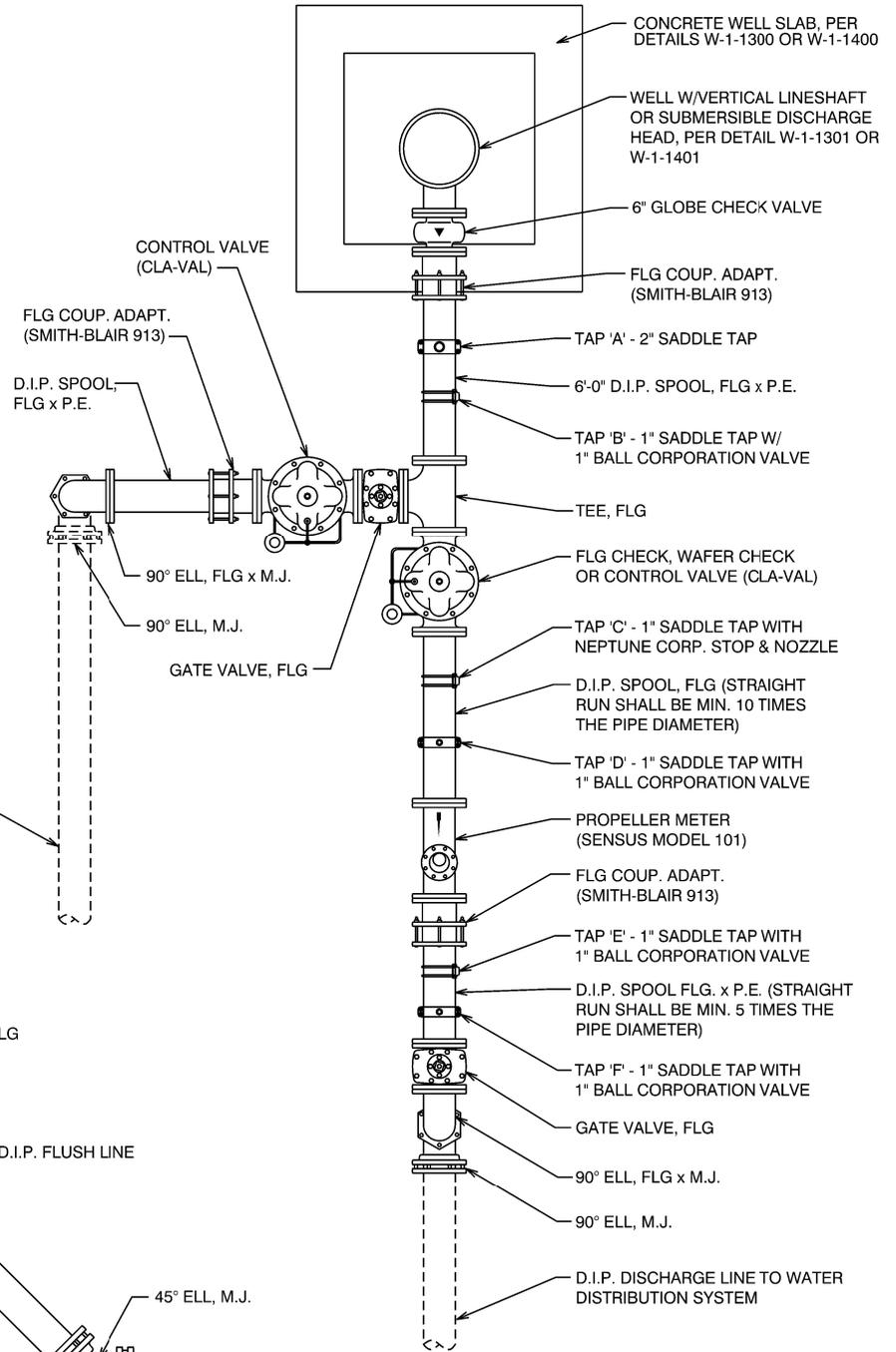
D.I.P. FLUSH LINE TO OPEN DISCHARGE AT CATCH BASIN, RETENTION BASIN OR DRAINAGE DITCH (SEE DETAIL BELOW)
