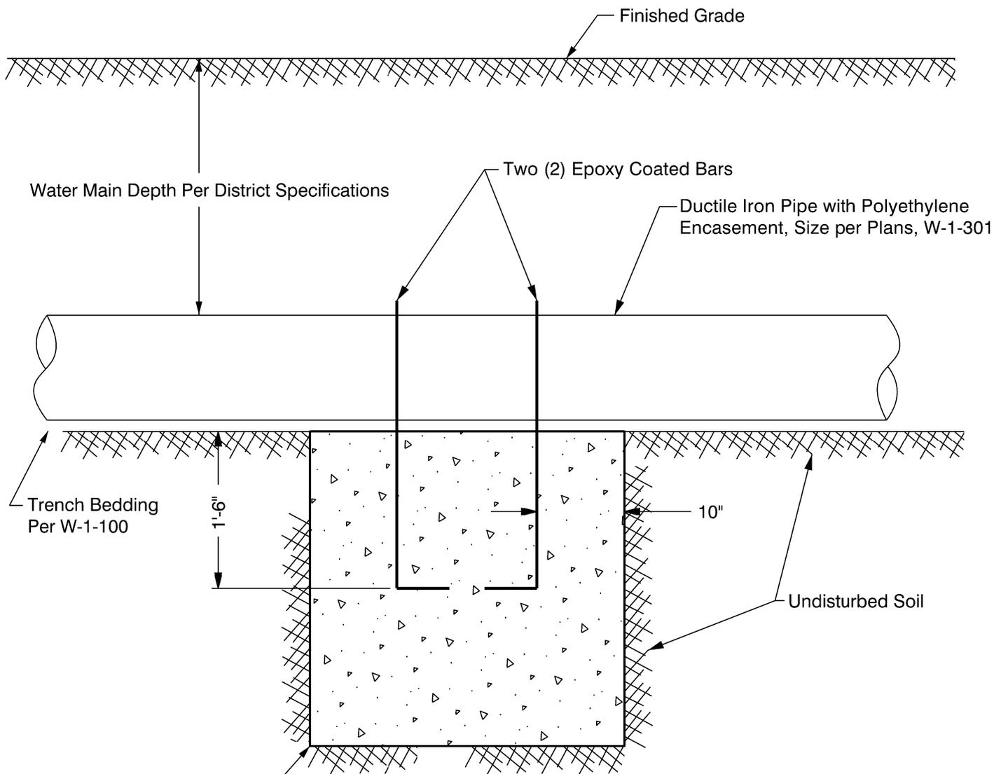
Min. Class "B" concrete, which is defined as concrete whose minimum compressive strength at 14 days reaches 2000psi and at 28 days reaches 2500psi. per MAG Section 725, Table 725-1.
