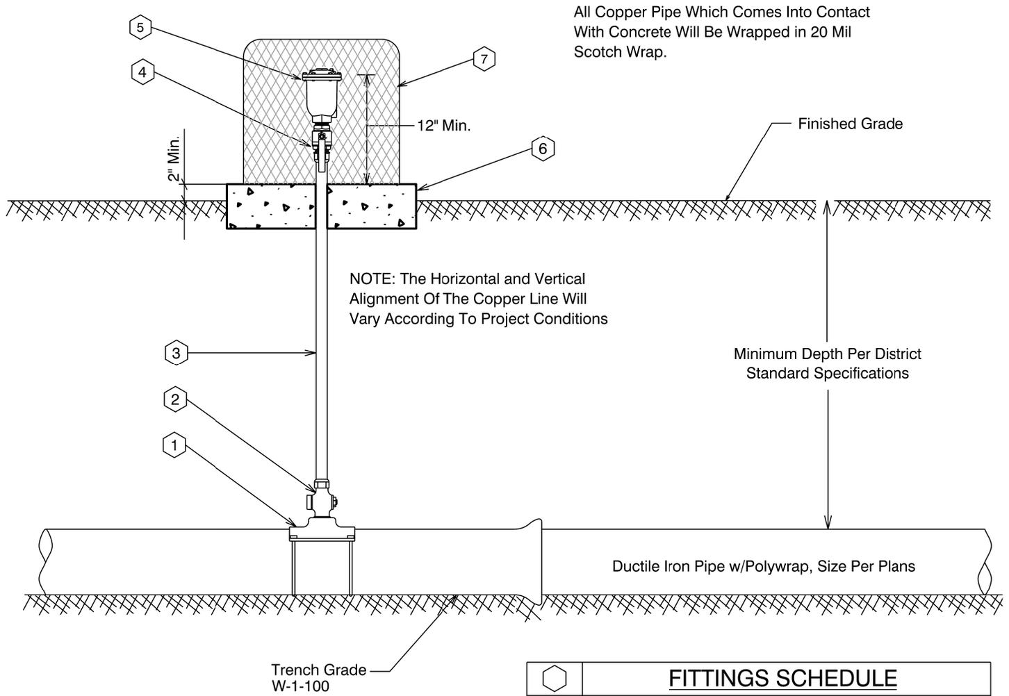
All Copper Pipe Which Comes Into Contact With Concrete Will Be Wrapped in 20 Mil Scotch Wrap.
