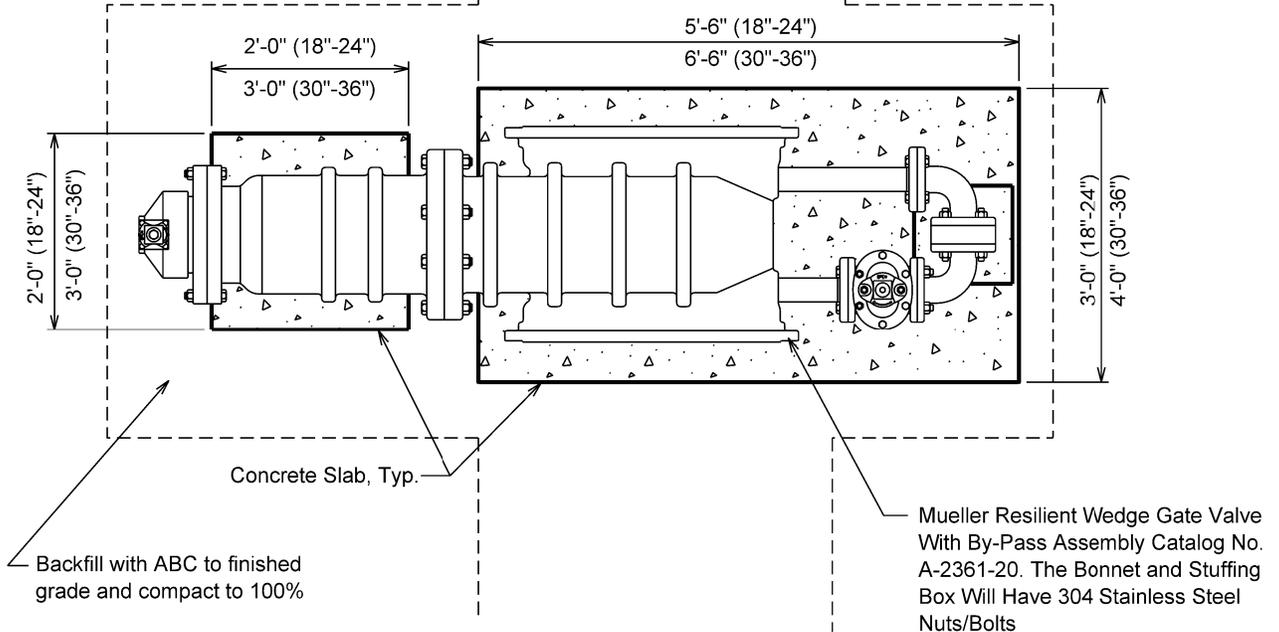
All concrete slabs to be class "C", which is defined as concrete whose minimum compressive strength at 14 days reaches 1600psi and at 28 days reaches 2000psi. per MAG Section 725, Table 725-1. Slabs to be formed and poured prior to valve installation.
